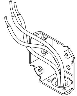
Position the body over the J Box and Secure the back plate to the wall
