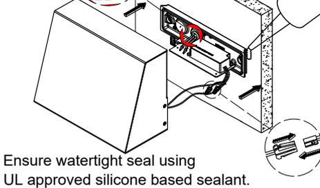
Ensure watertight seal using UL approved silicone based sealant.
